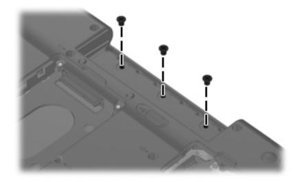
Where used: 3 screws (in the battery bay) that secure the top cover to the base enclosure
